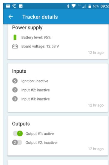
When switched to 'ON', the relay switched-circuit is open (vehicle immobilised).
