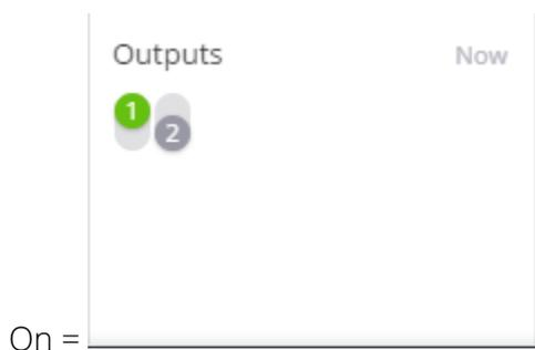
When switched to 'ON', the relay switched-circuit is open (vehicle immobilised).
