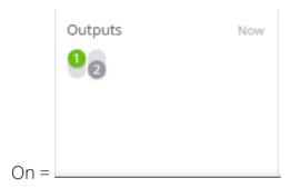
When switched to 'ON', the relay switched-circuit is open (vehicle immobilised).
